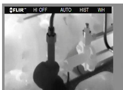
Figure 1: IR Camera View of Fugitive Emissions
