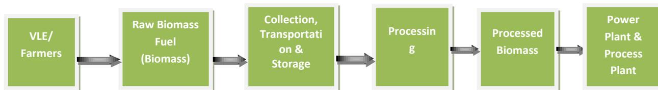
Figure 1: Flow Diagram of Biomass Supply Chain Management [2]
